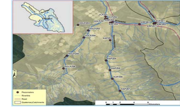
Figure 2: Twenty-one installed piezometers: 6 in Hol River, 7 in Krom Antonies River, 5 in Kruismans River, 2 Verlorenvlei River.
