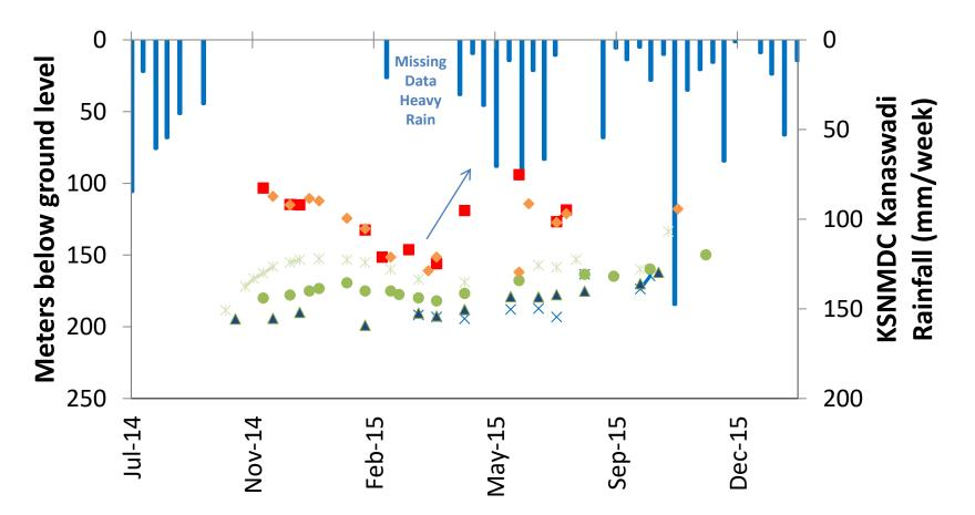
Participatory groundwater monitoring wells respond to rain => Rainfall recharge is definitely reaching deeper fractures.
