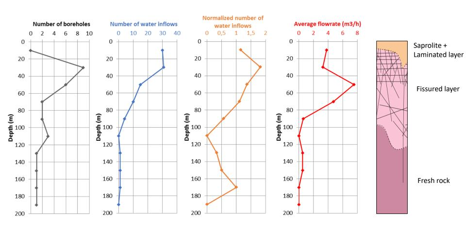
Blow flowrates of 26 boreholes (Air rock hammer drill)
