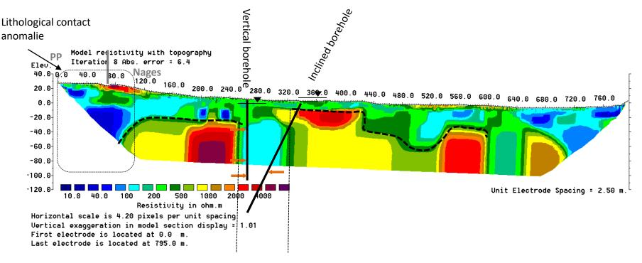
> Mineralised water in « deep » fissure network: greater resistivity contrasts
