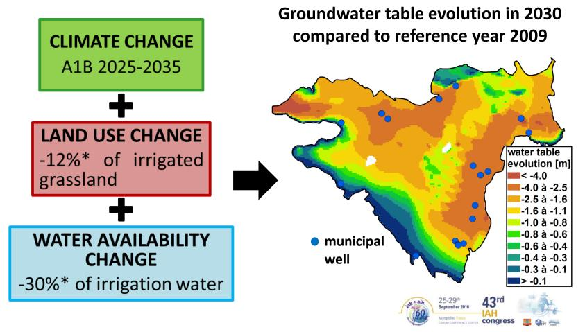
Development of a numerical model to simulate global change impact on the groundwater resource (ASTUCE&TIC / SIRRIMED)
