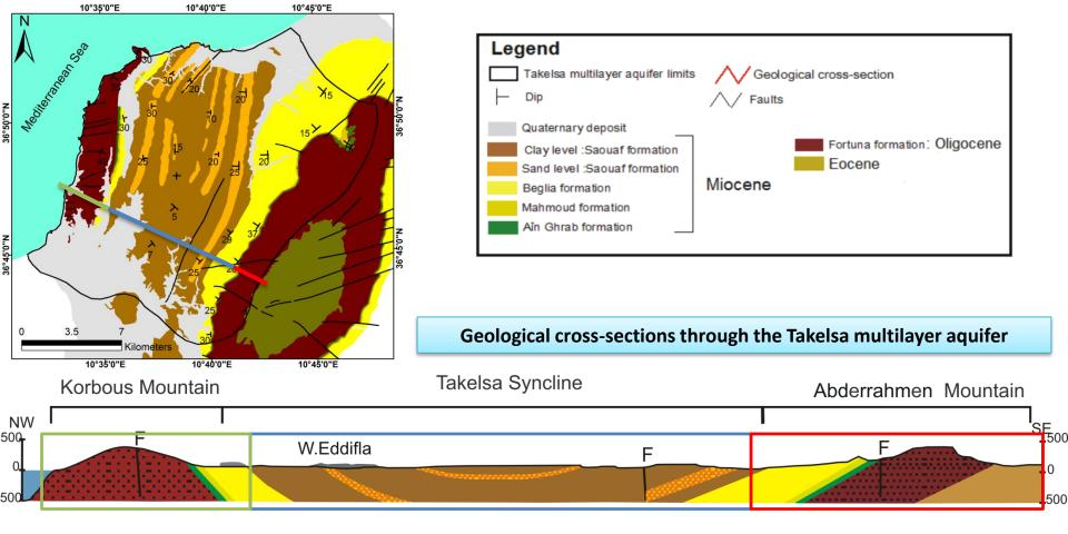
The Takelsa multilayer aquifer is mainly constituted by sandstone and clay series, dated from Oligocene to Quaternary ages. And the sandstone levels are exploited as aquifers. This aquifer is recharged by precipitation through the infiltration process in the permeable outcrops of sandstone.
