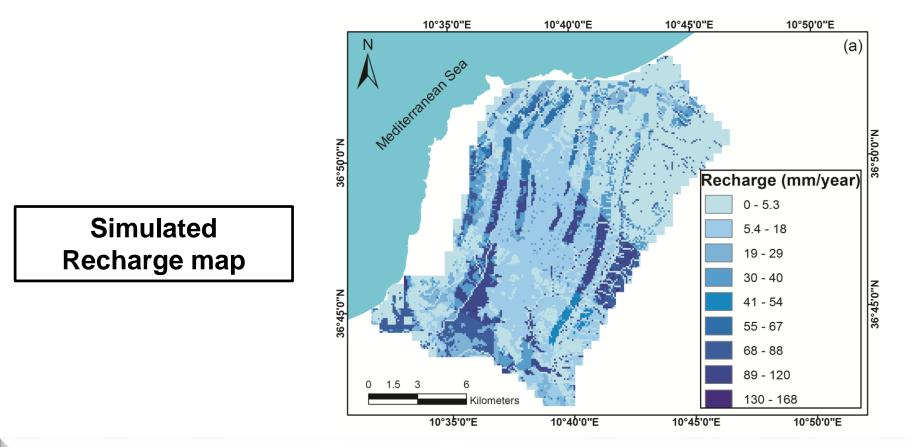
The groundwater recharge rate ranged from 0 to 168 mm/year with a mean value of 22 mm/year. The high values were observed in areas characterized by sandy loam and loamy sand soils, low slope and with intense vegetation cover.
