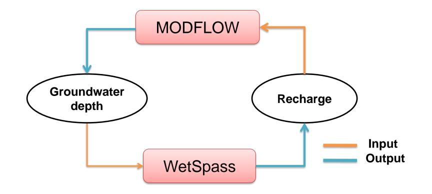
**MODFLOW** was used for the groundwater flow modeling. It resolves the flow equation by using the finite difference method in the steady and the transient states for multilayer aquifers.
