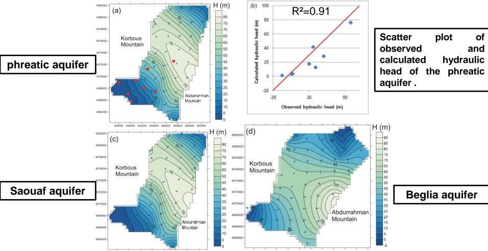
For the phreatic aquifer, the calculated hydraulic heads in steady state fit well to the observed ones
