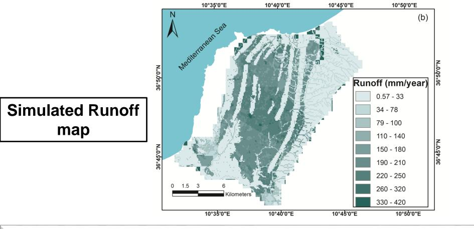
The surface runoff varied between 0.6 and 418.3 mm/year with an average value of 92 mm/year. The runoff is less accentuated in the Mountain areas. It is due to the high slope values and the presence of the shrub and the orchard associated with sandy loam and loamy sand soils. The omnipresence of agricultural land in the synclinal and the sandy clay levels with low slope reproduce high surface runoff.
