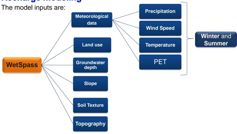
The groundwater recharge is calculated by considering the results of the water balance:
