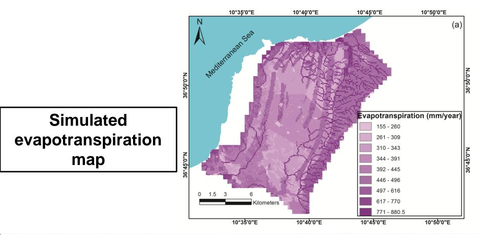
The evapotranspiration values obtained ranged from 155 to 880.5 mm/year with a mean value of 461 mm/year. High values are observed especially in water courses and forests areas characterized by sandy loam and loamy sand soil.
