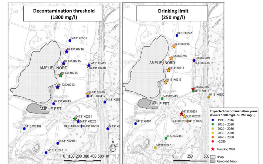
**Figure 5 : Predictive maps of decontamination for the thresholds of 1800 mg/l and 250 mg/l**
