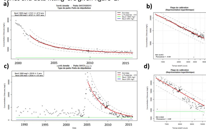
**Figure 2 : Example of chloride times series recorded at some pumping wells (black) with power law fitting (red) for different heaps. b) and d) graphs represent the fitting period on a log-log scale**
