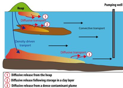
**Figure 1 : Conceptual model of contaminant storage and release**
