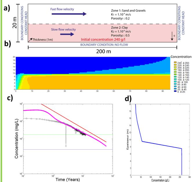
**Figure 4 : Release of dense contaminant from a low permeability layer to a high transmissivity layer with: a) the simulated configuration, b) the concentration distribution, c) the resulting BTC curve (Purple), the power law (red) and the data (black), d) the vertical concentration profile**
