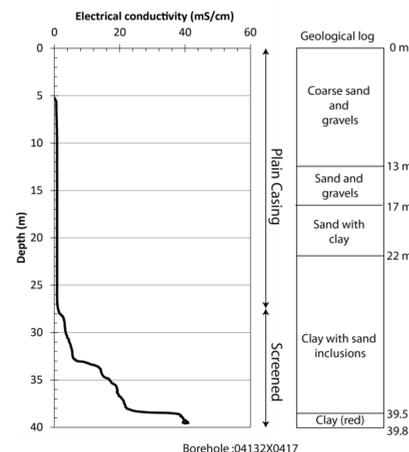
**Figure 3: Electrical conductivity log and geological log showing stratification of the contamination**
