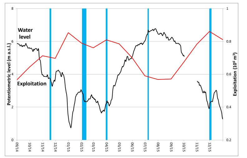
Five surveys during periods of higher and lower exploitation are performed to monitor the potentiometric level, the water temperature and the exploited flow rate.
