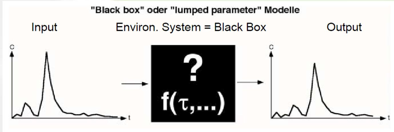
$$C_{out}(t) = \int_0^{\infty} C_{in}(t - t') \underbrace{\exp(-\lambda t')}_{\text{Decay of radioactive tracer}} \underbrace{g(t')}_{\text{Age distribution functions}} dt$$
