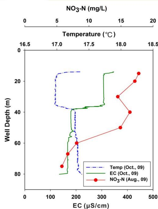
Leakage of perched GW : elevated NO<sub>3</sub>-N (14–18 mg/L) in the upper 50 m of well depth
