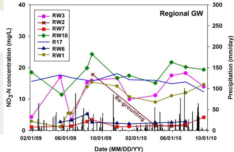
NO<sub>3</sub>-N concentrations at the RW2 : 17.8 mg/L → 1.5 mg/L before and after re-grouting.
