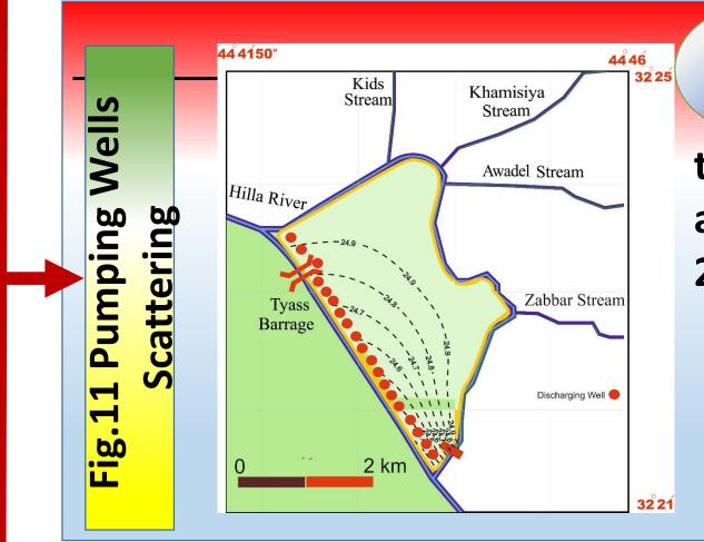
Hydrologic Solution a) It was planned to supply a net WD Col.4, Table.1 by a SW from Hillah River after adding 20% of WD, Col.5. B) Discharging the additional 20%WD in Col.6 by discharging wells of 4.6L/s discharging capacity scattering along Hillah River embankments Fig.11.
