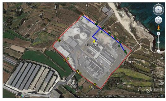
Water Level and Electrical Conductivity are the selected monitoring indicators. Monitoring undertaken through OTT Eco-Log probes installed in boreholes.
