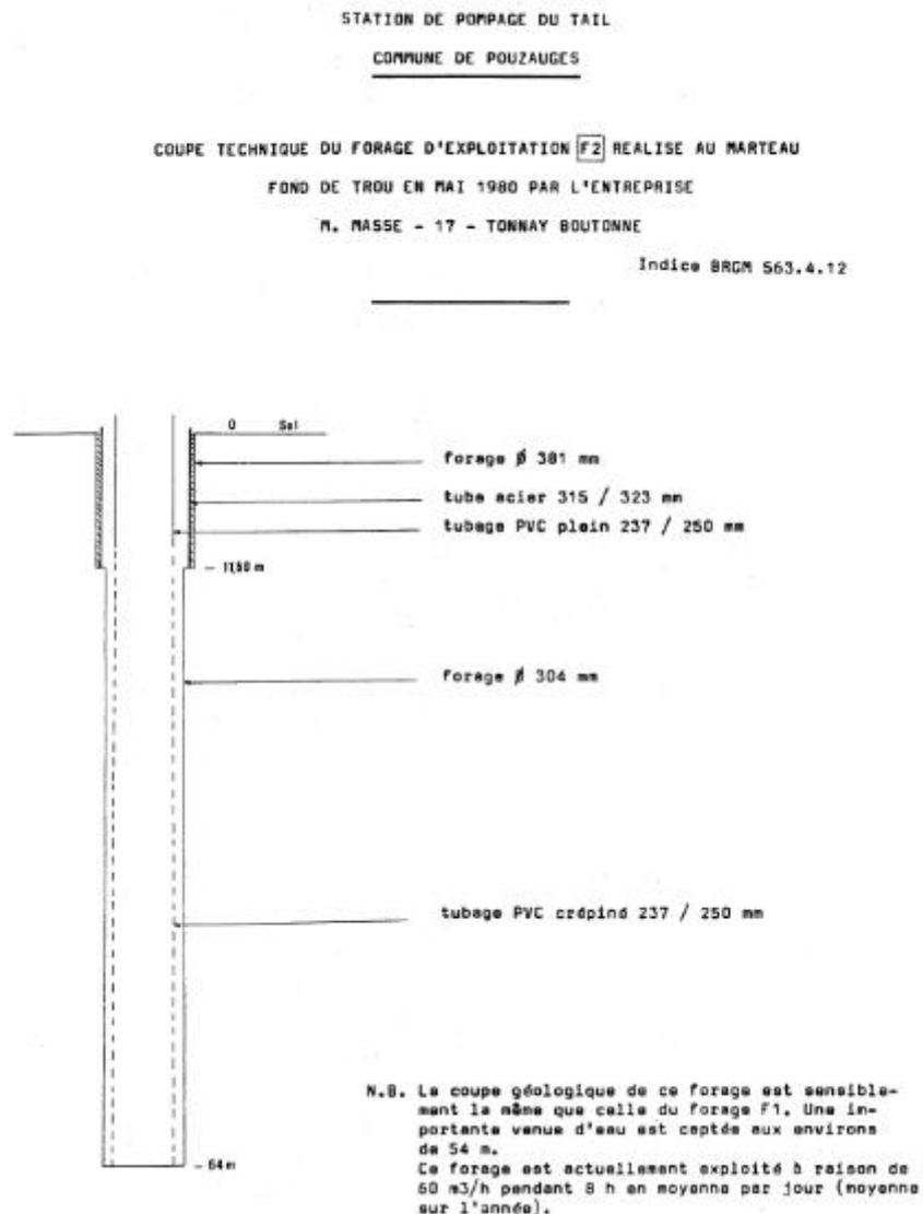
Figure 20 – Drilling log, borehole F2 (05634X0012/F2)
