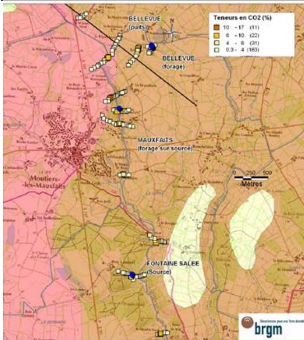
Figure 31 - Soil CO2 (September 2008 survey)
