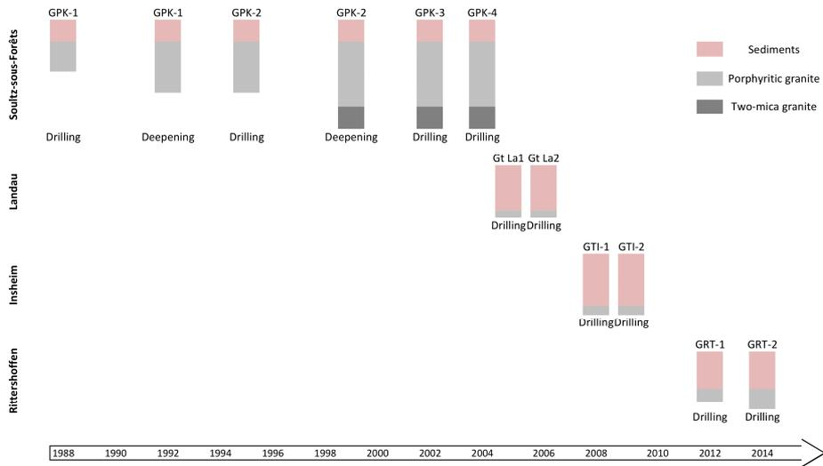
Figure 2 - Chronology of geothermal projects and associated deep wells in the Upper Rhine Graben
