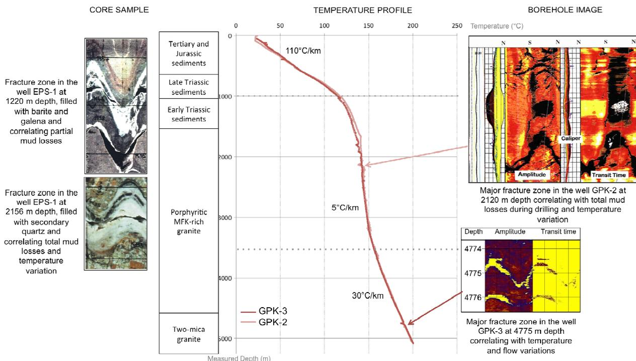
Figure 3 - Borehole images of major fracture zones in the geothermal wells GPK-2 and GPK-3 associated with thermal anomalies. Example of fracture zones from cored well EPS-1.
