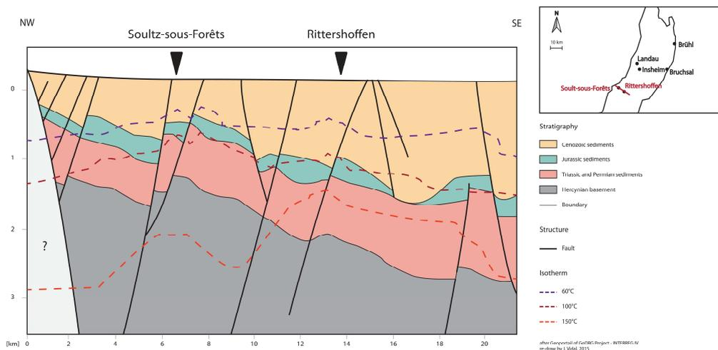
Figure 3 - Geological interpretation through Soultz-sous-Forêts and Rittershoffen geothermal sites
