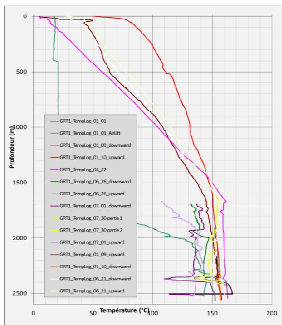
Figure 4 - Temperature logs in GRT-1. Depths are given in MD
