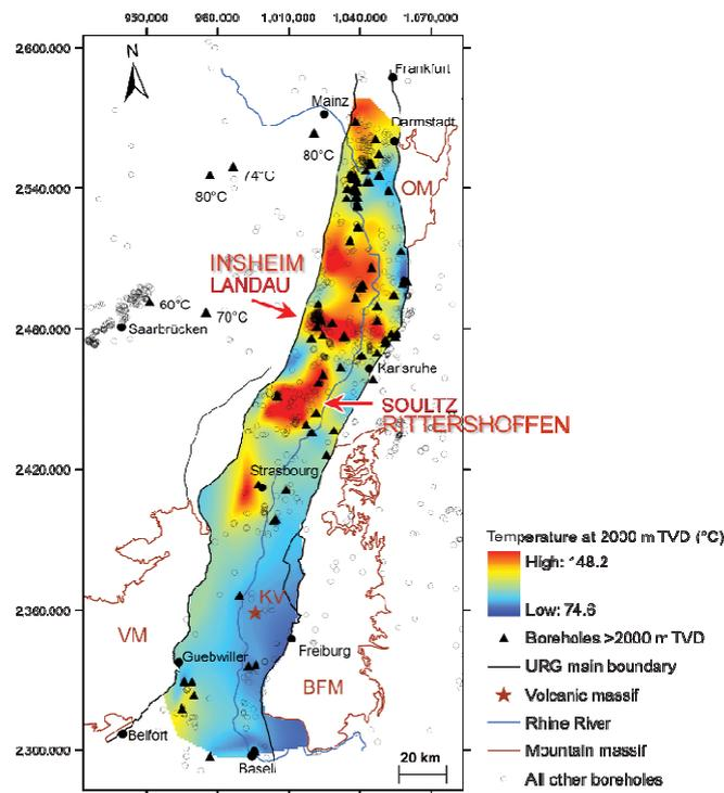
Figure 1 - Temperature distribution at 2000 m depth in the URG (Baillieux et al., 2013)
