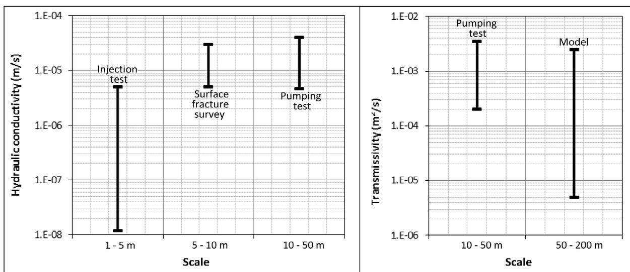
Figure 3 – Hydraulic parameters and scale of measurement of the different methods used.
