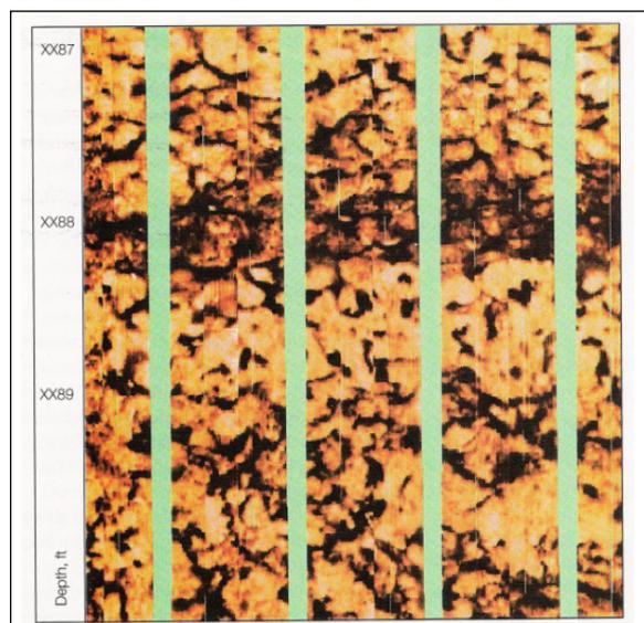
Figure 8: Mottled fabric of a Middle-East carbonate rock shown by a FMI image (dark = pores, light = grains and matrix).
