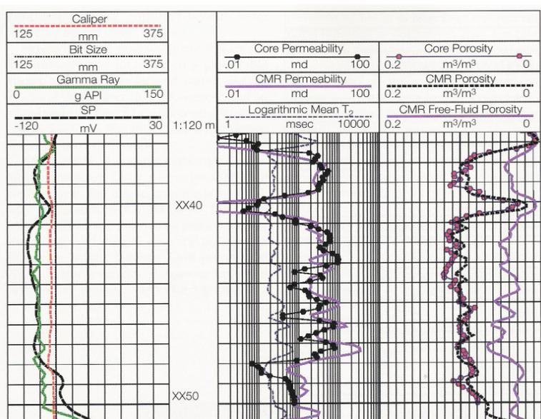
Figure 6: Comparison of CMR porosity and CMR permeability with core measurements.
