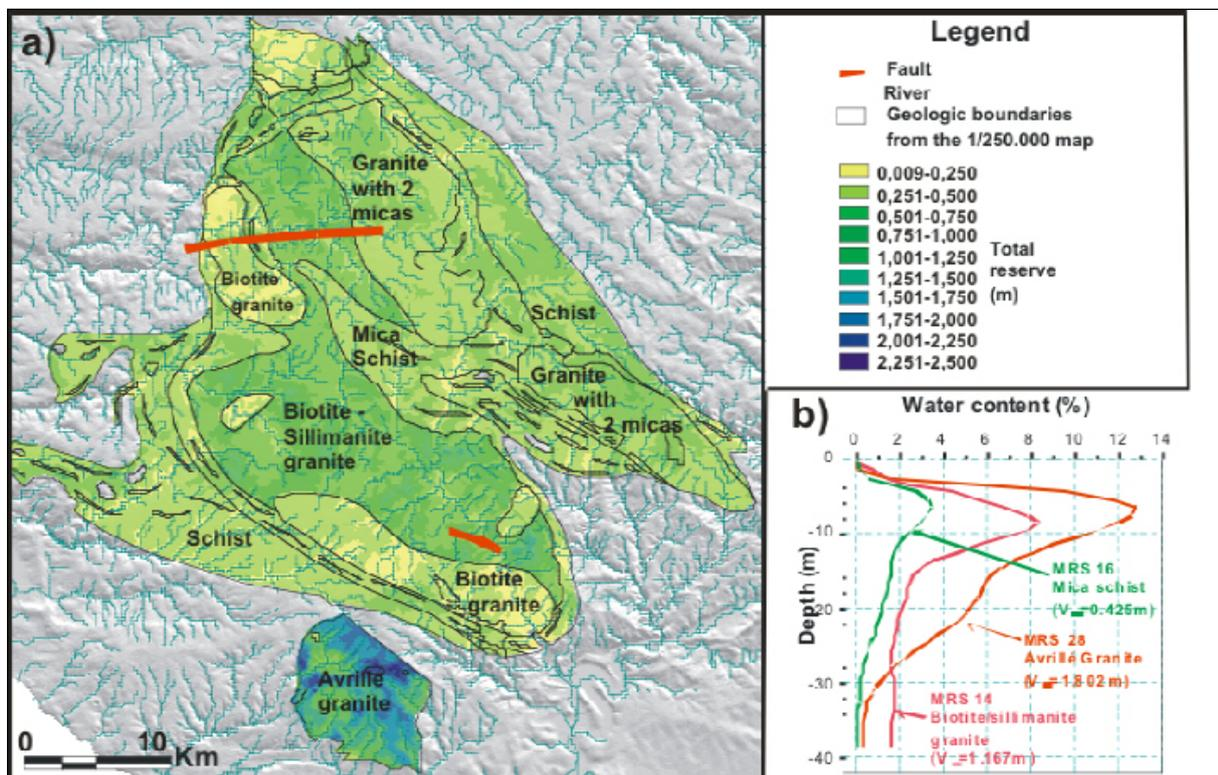
Figure 6: La Roche-sur-Yon region: a) Thickness map of total reserves in the weathered aquifers. b) Example of MRS water content profiles measured in different geological settings.
