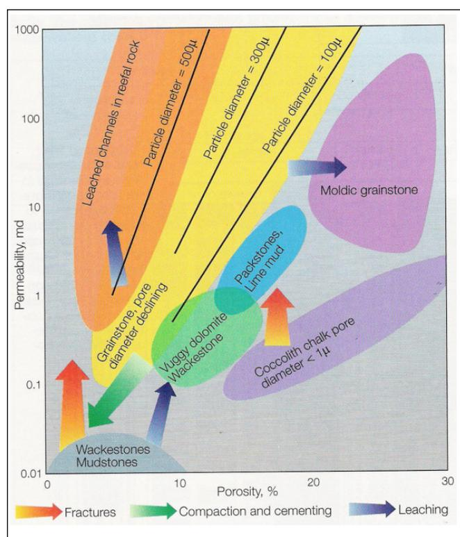
Figure 2: Porosity, pore type, and permeability in carbonates.
