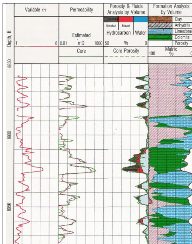
Figure 3: Comparison of "variable m" permeability and core permeability, in a Middle-East carbonate.
