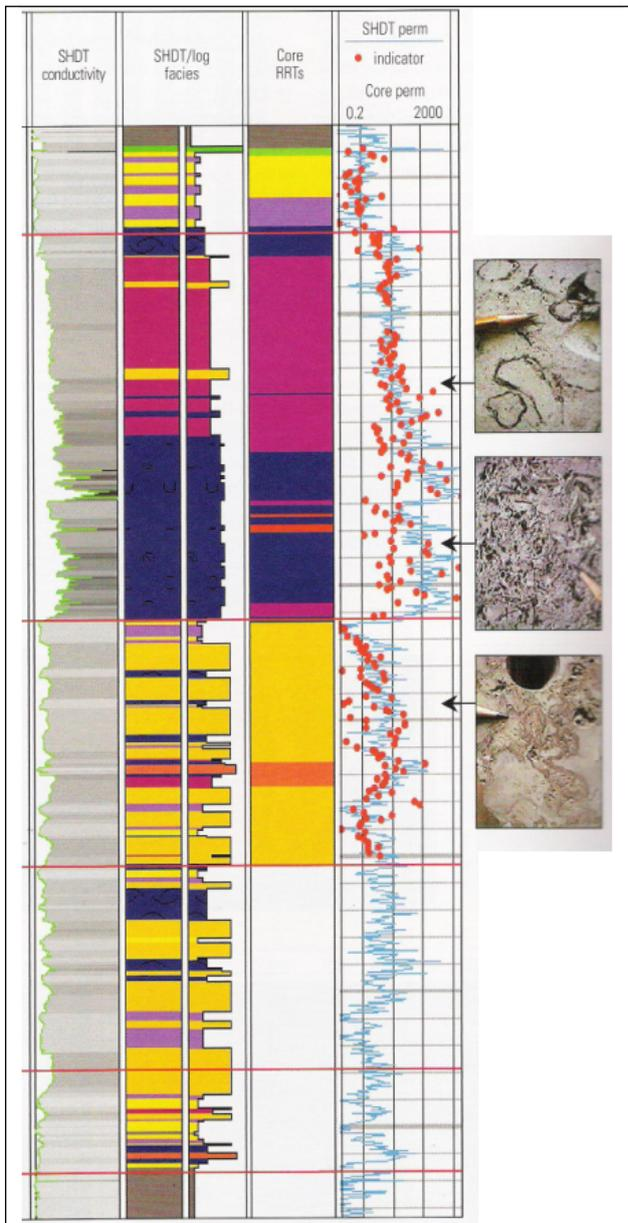
Figure 9: Rock type zonation and continuous permeability indicator derives from high-resolution dipmeter data combined with conventional porosity and lithology logs.
