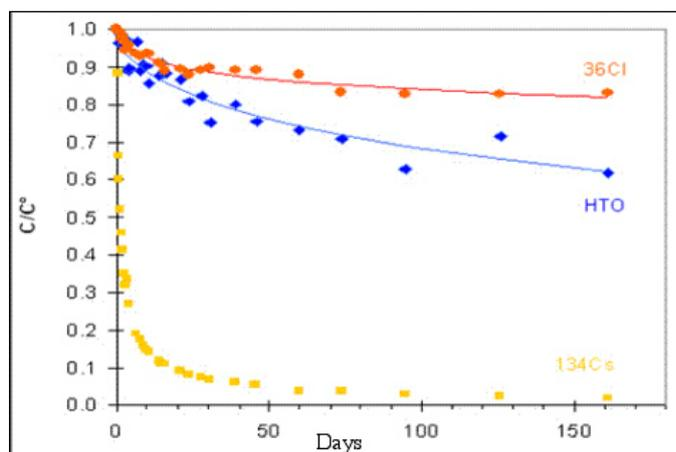
Figure 5: Evolution of tracer concentration in a diffusion borehole showing three behaviours: water (HTO), cationic retention ( $^{134}\text{Cs}$ ) and anionic exclusion ( $^{36}\text{Cl}$ )
