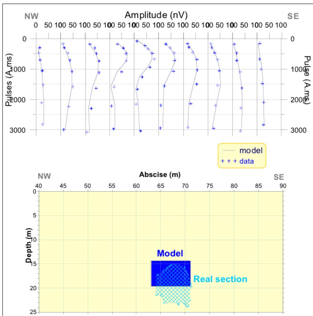
Figure 7: Karst conduit imaging near Pou Meyssen (France). 10 MRS were performed along a profile crossing the conduit. Data curves (top) were simultaneously inverted to obtain a 2D model (bottom)
