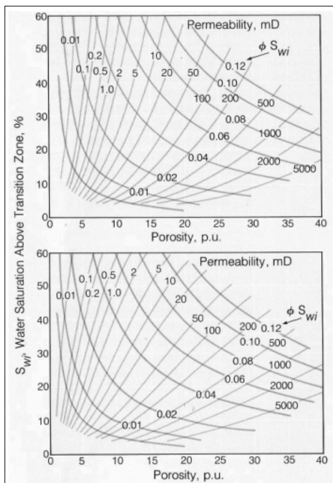
Figure 1: Charts based on permeability transforms proposed by Timur (top) and by Wyllie and Rose (bottom).
