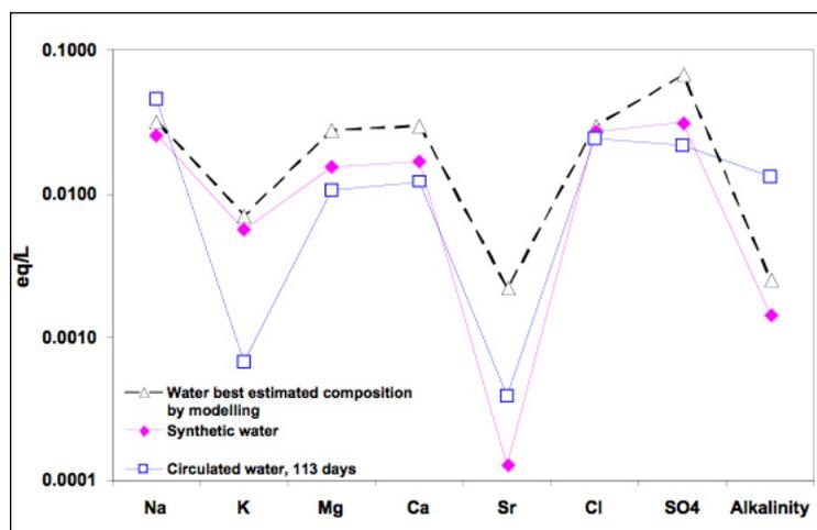
Figure 4: Pore water chemical composition obtained after 113 days of water circulation
