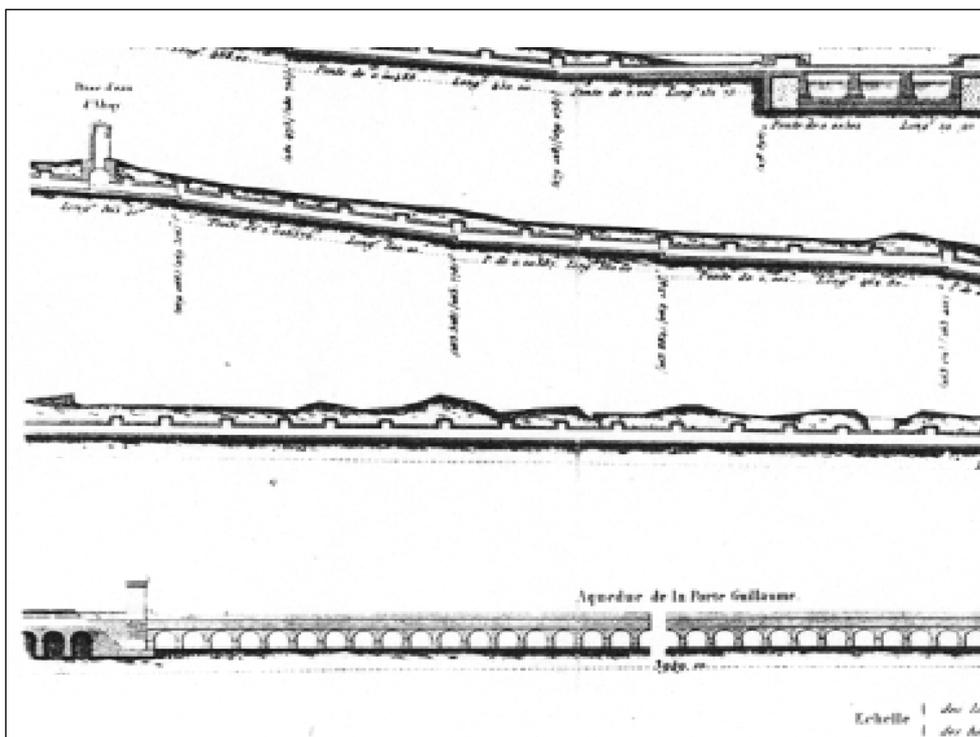
Figure 1. Profile of the Aqueduct that conveys the Rosoir Spring water to Dijon, Plate 2.
