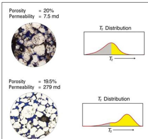
Figure 5:  $T_2$  distributions for two sandstones with same porosity but different permeabilities and pore sizes (the yellow area corresponds to free-fluid porosity).
