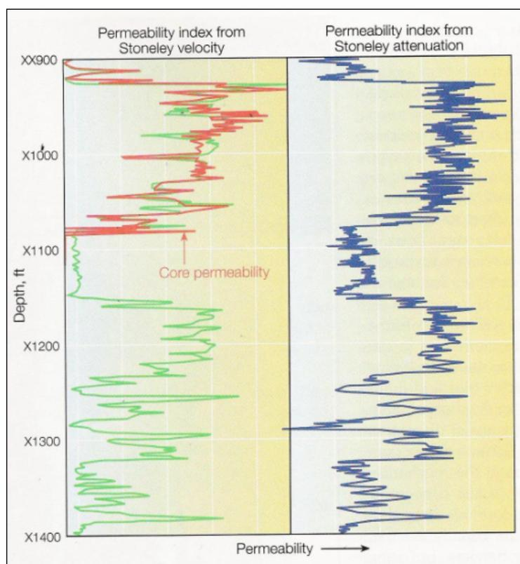
Figure 4: Comparison of core measurements and permeability indexes from Stoneley waves, in a Middle-East carbonate.
