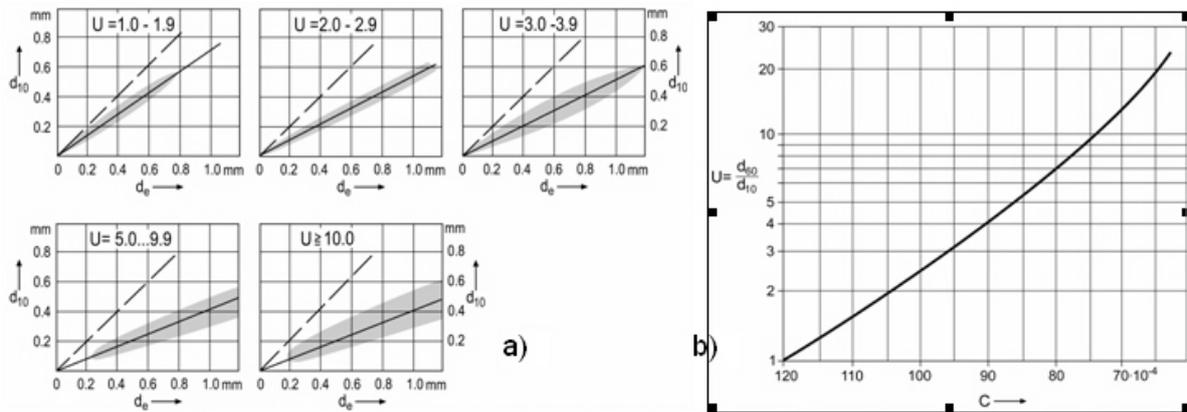
Figure 2: a) Relation between  $d_e$  and  $d_{10}$  for different ranges of  $U$ ; b) Factor  $C$  as function of  $U$  (modified after Beyer 1964)
