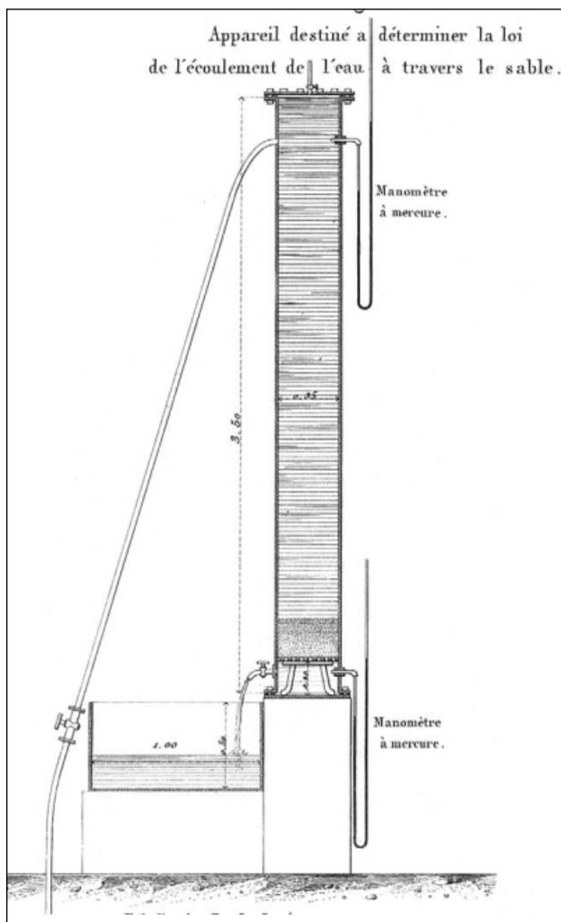
Figure 4. Darcy’s original sand column apparatus (Darcy 1856, Plate 24, Figure 3).
