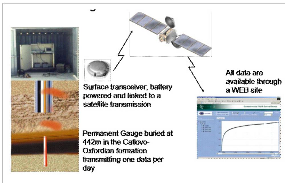
Figure 7: General set up of an electromagnetic pressure monitoring system
