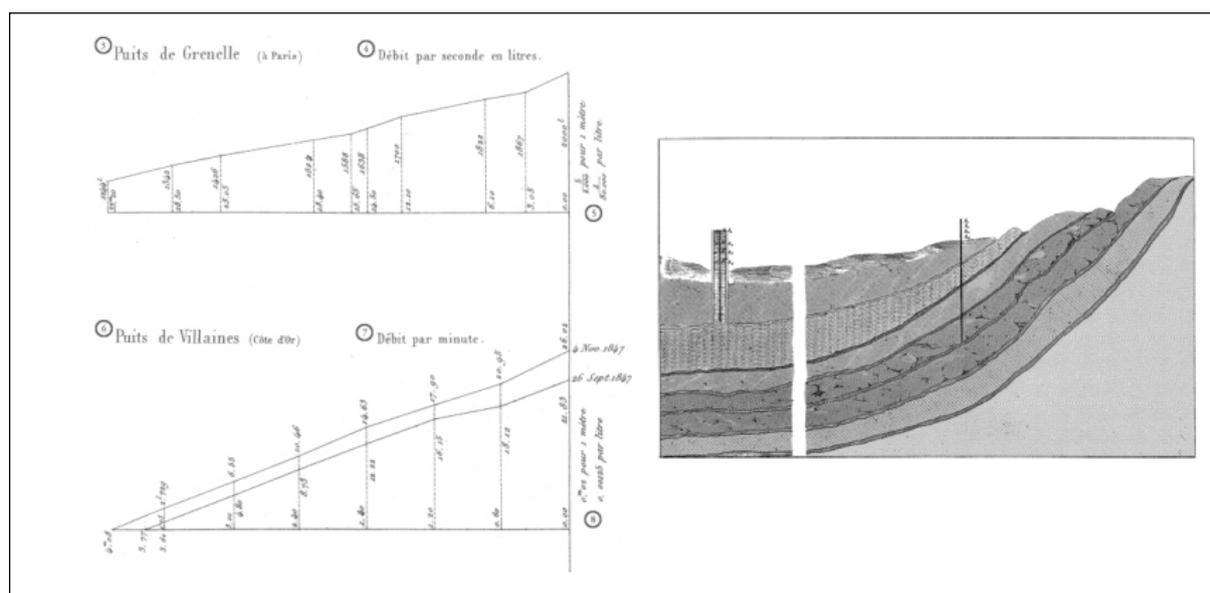
Figure 5. Darcy's measurements of artesian spring flow and his linear observations (Darcy 1856, Plate 22).
