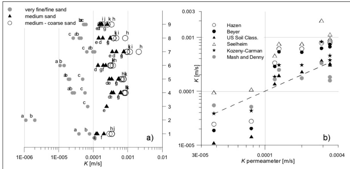
Figure 3: a) K-values for 11 samples from permeameter (1), infiltration (2), borehole dilution (3) tests and after empirical methods Hazen(4), Beyer(5), US Soil Classification (6), Seelheim (7), Kozeny-Carman (8) and Mash-Denny(9); b) All methods compared to permeameter results (1 : 1 line)
