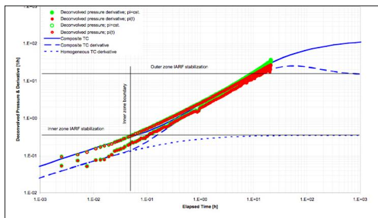
Figure 8: Interpretation of a short term pulse test
