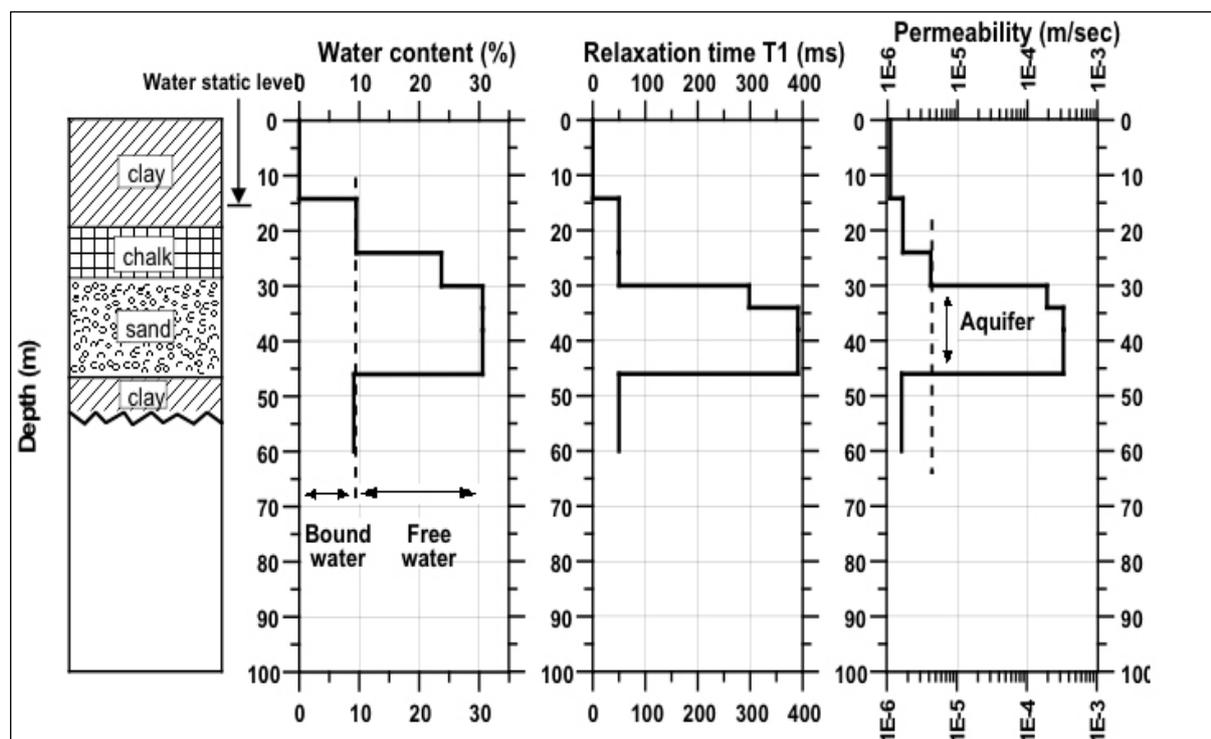
Figure 1: Borehole information and MRS results near Chuignes (Beauce, France) studied site (transmissivity is  $4.7 \cdot 10^{-3} \text{ m}^2/\text{s}$ , with a similar estimation from pumping test and MRS)
