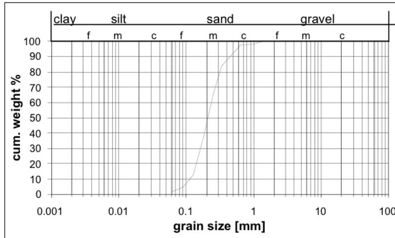
Figure 1: Example of a cumulative grain size distribution curve for a fine to medium sand
