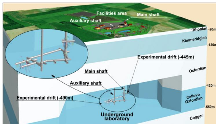
Figure 3: General layout of the underground drifts of the Bure URL
