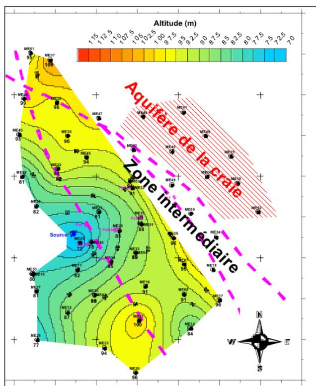
Figure 2: Water table elevation mapping using MRS over the “Cuisien” sand aquifer catchment of Montreuil-sur-Epte (Paris Basin)
