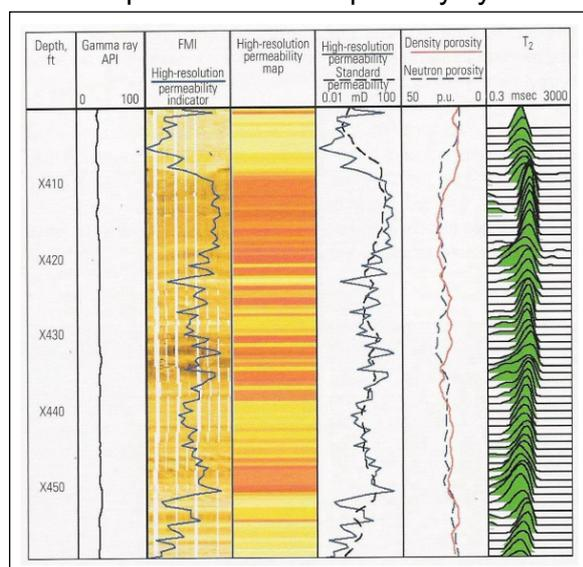
Figure 7: Comparison of CMRPlus high-resolution permeability with FMI borehole electrical images
