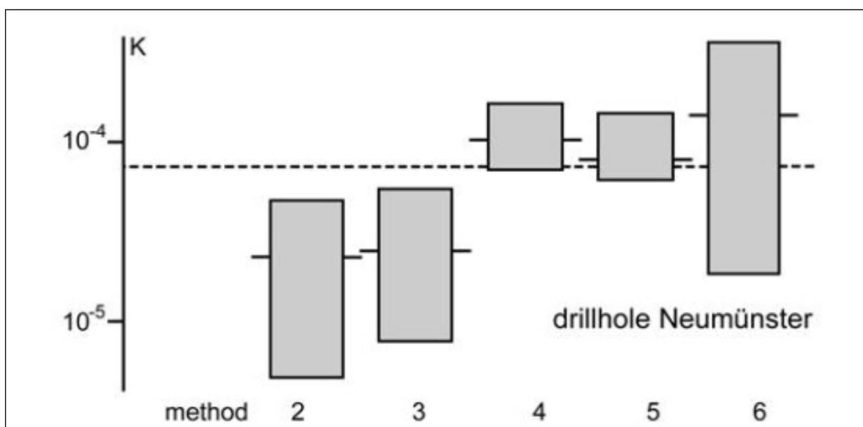
Figure 4: Comparison of permeameter tests, flow downwards (2) and flow upwards (3), Hazen (4) and Beyer (5) and pump test results (6) (modified after Pekdeger and Schulz 1975)
