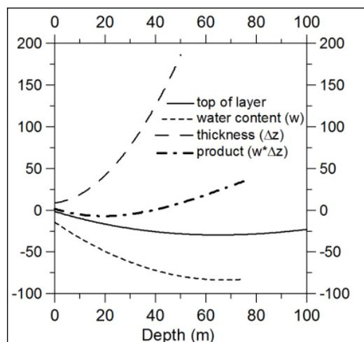
Figure 5: Numerical study of MRS parameters resolution (from Legtchenko et al., 2004). Signal of a 10 m thickness layer with 20% of water content was modelled for a 100 m square loop. Inversion provides top of layer, water content (w), thickness (Dz) and product (w\*Dz). Error on parameter P is estimated as:
