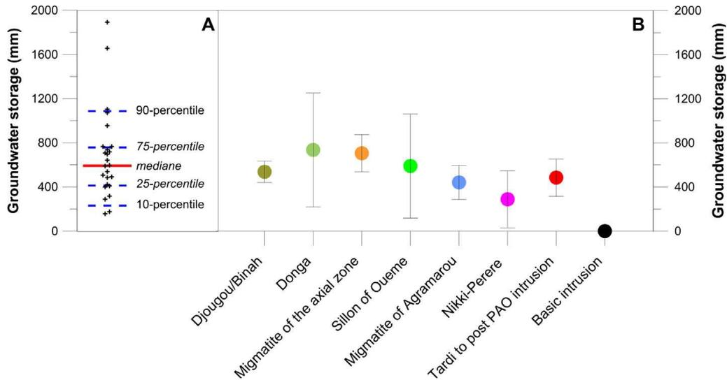
Figure 4 – Groundwater storage in hard rocks in the study window (from Vouillamoz et al., 2015). A: Percentile. B: Variation of storage among geological units (the point is the median value and the error bars are the mean difference to the median).
