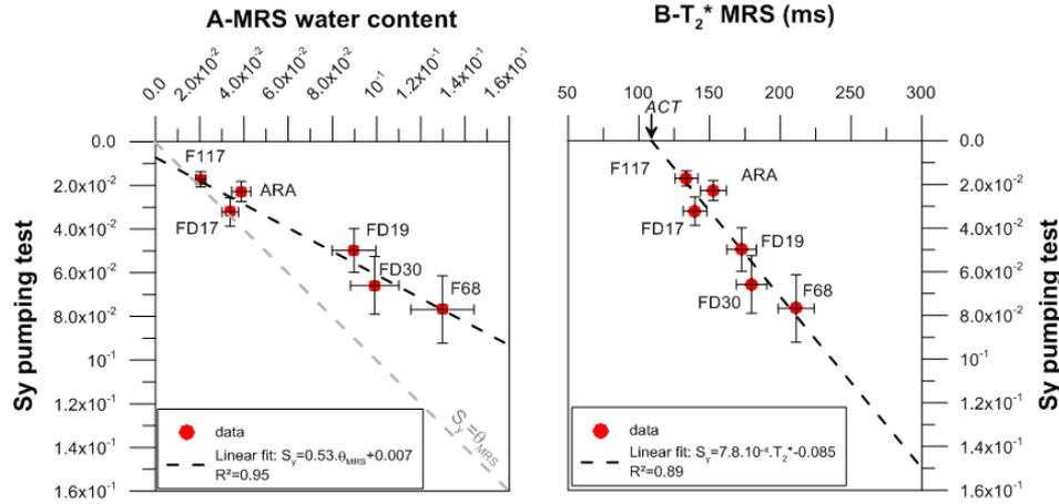
Figure 3 – Comparison of MRS parameters with specific yield.  $R^2$  is the coefficient of determination. A: MRS water content. B: MRS decay  $T_2^*$  (from Vouillamoz et al., 2014).
