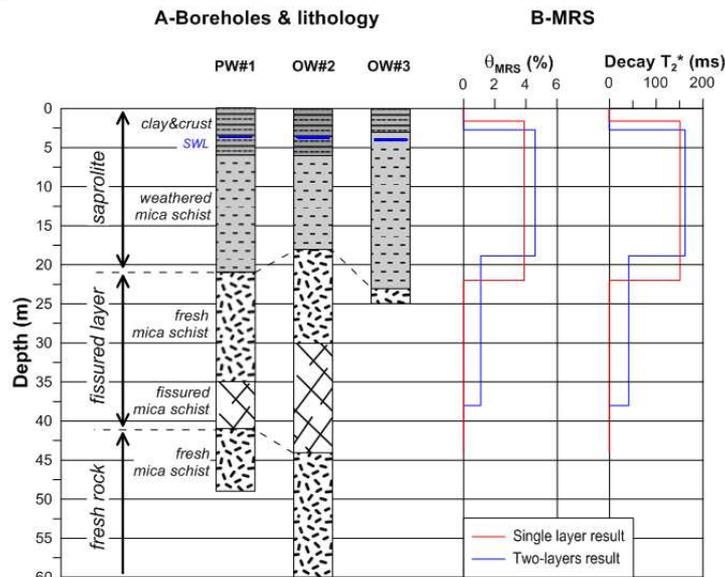
Figure 5 – Experiments at ARA site. A: Borehole lithology. SWL is the static water level. B: MRS results (modified from Vouillamoz et al., 2014).
