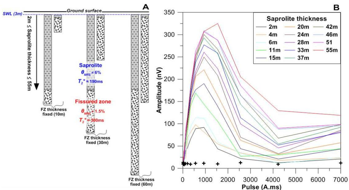
Figure 2 – Computed MRS models. A: Models geometry and input parameters (SWL is the static water level). B: Computed signals for a fixed FZ thickness of 30m. The crosses are the EM noise.
