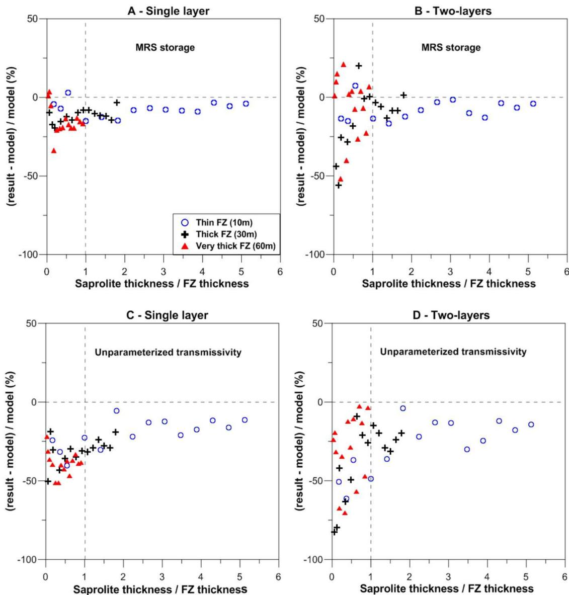
Figure 6 – Comparison of the MRS single and two-layer results to the initial model results. A&B: MRS storage. C&D: No-calibrated transmissivity.
