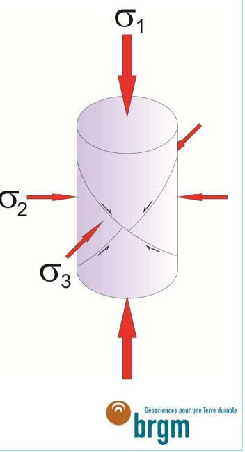
At the opposite, if we increase the confining stress  $(\sigma_1 = \sigma_2)$  while maintaining constant the third component  $(\sigma_3)$ , then we get a breaking by tension cracks, the cracks being parallel to  $\sigma_1$  and  $\sigma_2$ .
